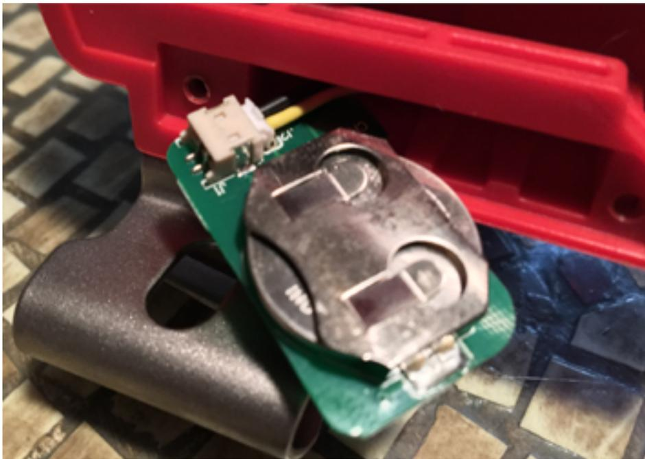
*Coin cell is behind a small panel that is underneath where the RedLithium battery attaches*
